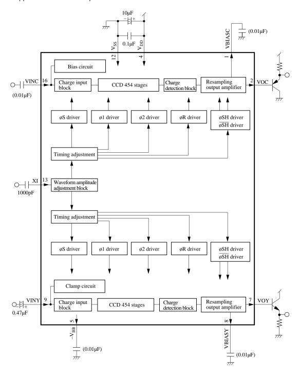
Note: If the external capacitor attached to pin 5 is an electrolytic capacitor, attach the negative pole to pin 5.
